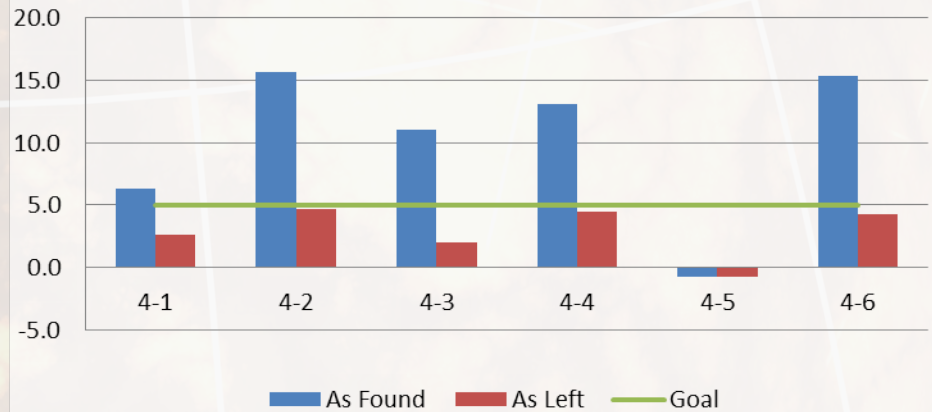
Primary Airflow - Measured vs Indicated (avg across load range)
